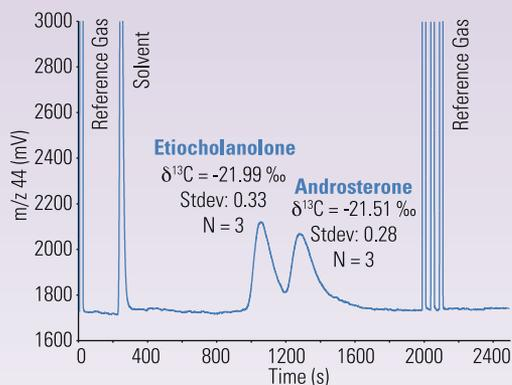
Analysis of steroids in urine (LC fraction) by high temperature HPLC coupled to IRMS.
