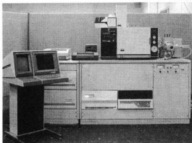
Figure 13. C 7 quadrupole GC/MS system, which did not go into production (1981).
