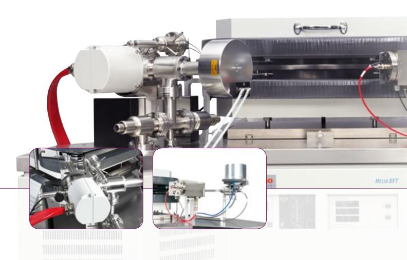
These temperature controlled evacuated amplifiers have an extended measurement range of 50 V, rather than the historical 10 V, giving the system an improved dynamic range.
